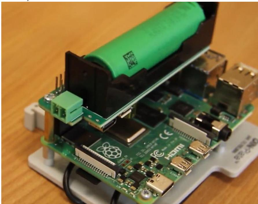
9. Plug the RTC and the platform on top of the watchdog, again use the correct pins. (Left most 6 pins (3 x 2) when the HDMI port of Raspberry Pi is facing you, right most end if you are looking at the header pins)
