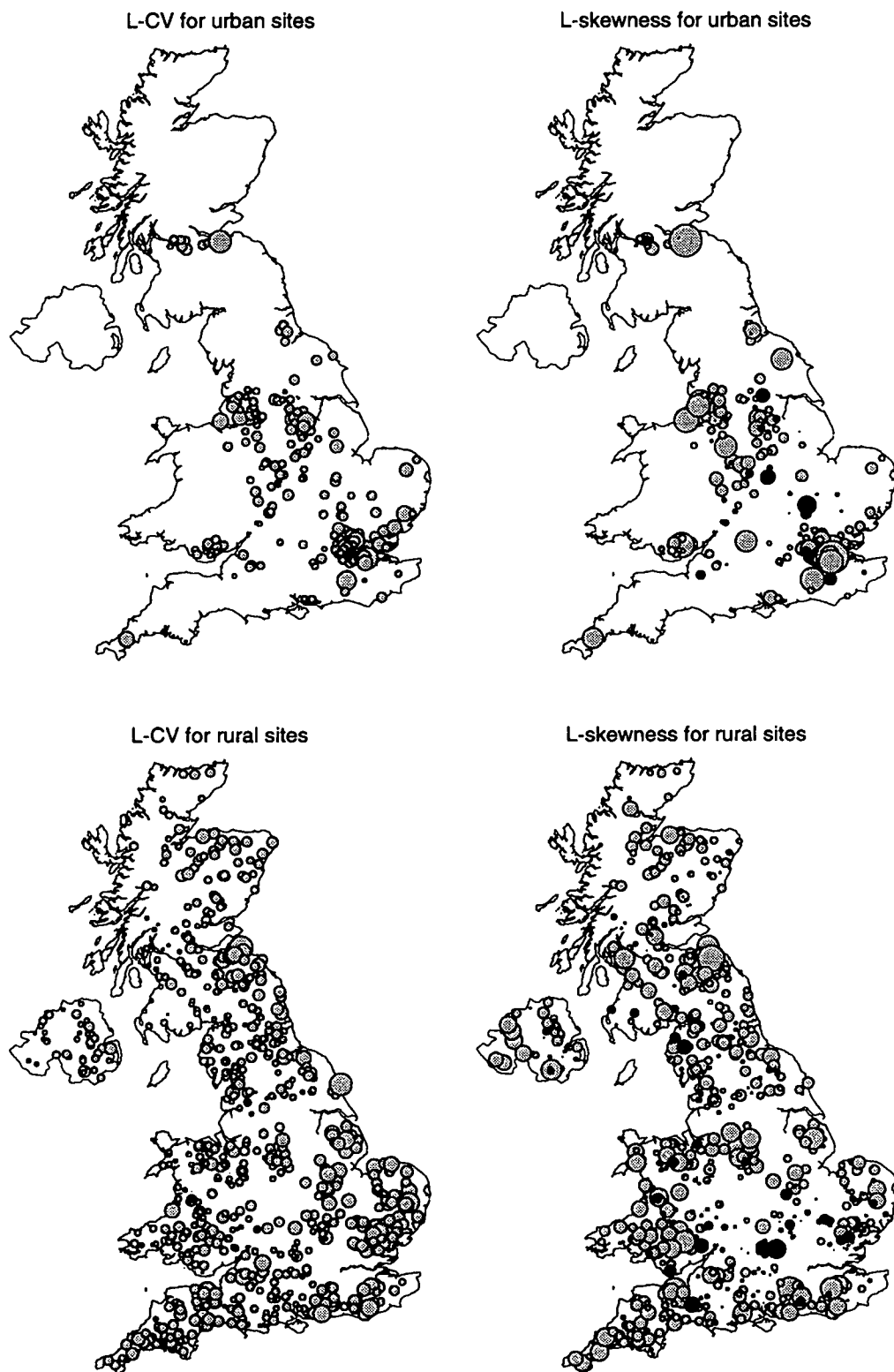
Figure 14.5 Maps of site L-moment ratios for urban and rural sites. Adjusted L-moment ratios are used for permeable catchments (§14.3.6). Grey circles show positive values, black circles negative. Note that L-CV is always positive.
