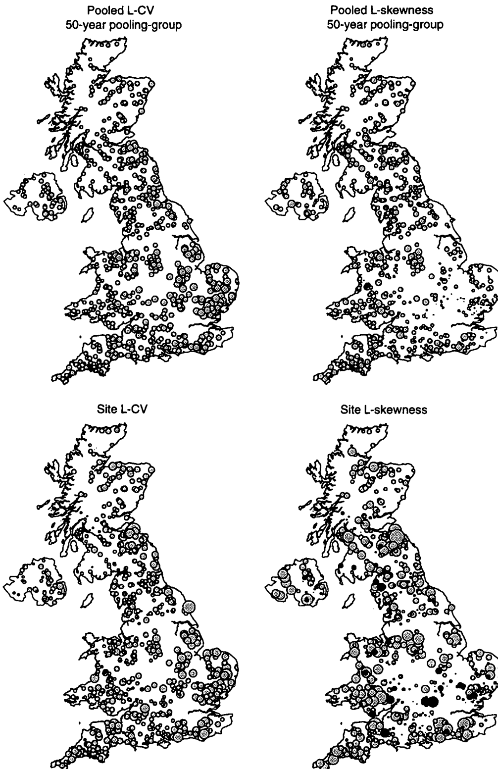
Figure 17.2 Maps of site and pooled L-CV and L-skewness for rural UK sites (positive values in grey, negative in black: N.B. L-CV values are always positive). Site and pooled L-moment ratios are shown to the same scale.
